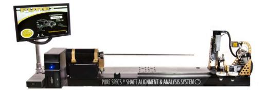
For each driver shaft, a *TaylorMade tip adapter* was installed with the neutral orientation 90 degrees from the PURE plane. The adjustable weights on the R15 head were left touching each other in the middle in the neutral position. Each six-iron shaft
